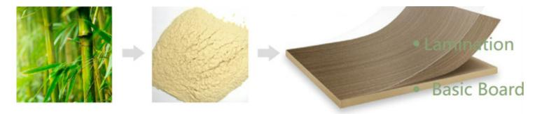
Modified bamboo wood fiber mixed with high molecular polymers.
